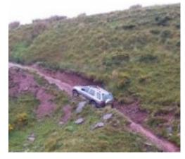
can't go up, better to reverse down. Handbrake on, clutch, into reverse, off clutch handbrake off. Check steering wheel is straight. Check behind is clear. Ignition off, then to on, then start engine and immediately we are driving backwards under control.
