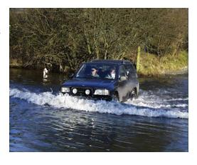
The preferred method of fording deep water is to travel at the same speed as the bow wave that forms in front of your vehicle. This phenomena creates a lower water level in the engine bay thus assisting in keeping it running.
